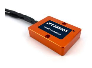
The Carrot Uego controller is capable of measuring the level of oxygen in the exhaust gas at high speed, in combination with a Bosch LSU4.9 lambda sensor. The controller is transmitting this data to the engine management system by CAN-bus or an analogue signal. The controller provides an accurate lambda measurement even when the exhaust gas temperature is changing rapidly.
